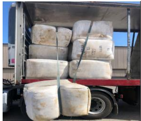
Photo 1. Incorrect loading of wool bales – the first two tiers were strapped lengthways rather than base out, across the truck. This arrangement resulted in an unstable load.
