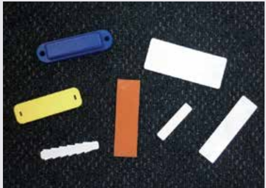
Examples of different RFID tag types tested to determine the "best performing"
