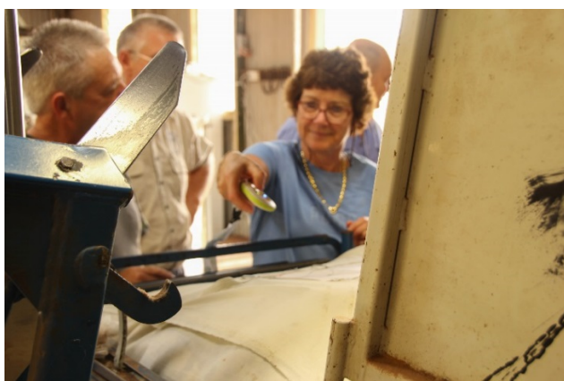
Photo 6: Scanning RFID Tag Id of bale in wool press
