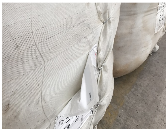
Photo 2: RFID tag adhered under a pack label
