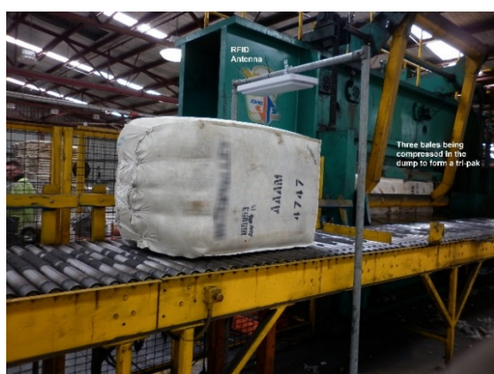
Photo 10: Bale passing under RFID antenna
